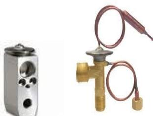
Expansion valves regulate the amount of liquid refrigerant flowing from the condenser to the evaporator based upon the evaporator pressure. A thermal expansion valve will include a temperature sensor and meters the amount of refrigerant flowing into the evaporator.
