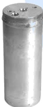
Air conditioning systems utilize a receiver drier to extract moisture from the system. The receiver drier is used on ac systems which make use of an expansion valve to control refrigerant flow and is located on the high-pressure side of the system, between compressor and the condenser. The receiver drier stores a portion of the system's refrigerant and contains a moisture absorbing substance to remove any moisture the system may become contaminated with.
