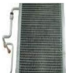
The ac condenser and your car's radiator often look quite similar in appearance. The compressor of the car generate compressed gas and sends it along to the top of the condenser, where the gas begin to cool. The gas continues to cool and condense as it makes its way through the serpentine-like coil arrangements, before exiting the bottom of the condenser as a high-pressure liquid. The condenser is usually located in front of your car's radiator.
